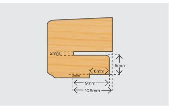
Automatically spaces the double glazed unit with a choice of 1mm to 6mm colour coded packer
