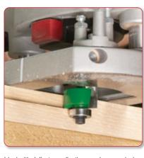
Ideal with delicate applications such as musical instrument production, when a small rebate is required for insertion of purfling.
