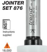
This Comb Jointing Set can be fitted to all heavy duty routers mounted in a fixed head position. It comprises a set of five 4mm kerf, TCT groovers, mounted on an arbor and three ball bearings. These offer alternative cutting depths and provide a self-guiding facility.
