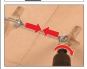
Turn hex bit to tighten Zipbolt and to tighten joint.
