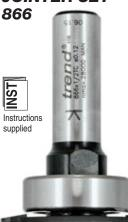
Ref. 866 Finger Jointer combines an assembly of five TCT slotting cutters with an abutting-edge cutter to produce a profile that extends the glue line threefold, resulting in an extremely strong joint. It fits into any portable or stationary router with a 1/2" collet.
