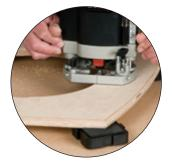
Routing with bottom clearance. Simply position blocks in corners.
