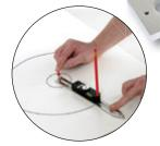
Compass Allows the drawing of circles with various diameters.
